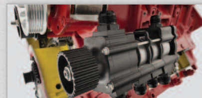
Mercury Racing Designed Dry-Sump Oil Pump
